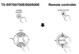
3. Press the ◀ and ► cursor buttons to set the desired level.
